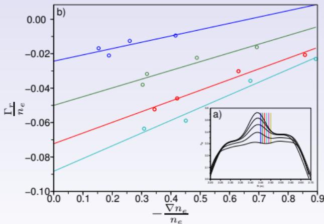
Knowing  $\Gamma_r(r, t)$  and  $n_e(r, t)$ ,  $D$  and  $V$  are calculated from :
