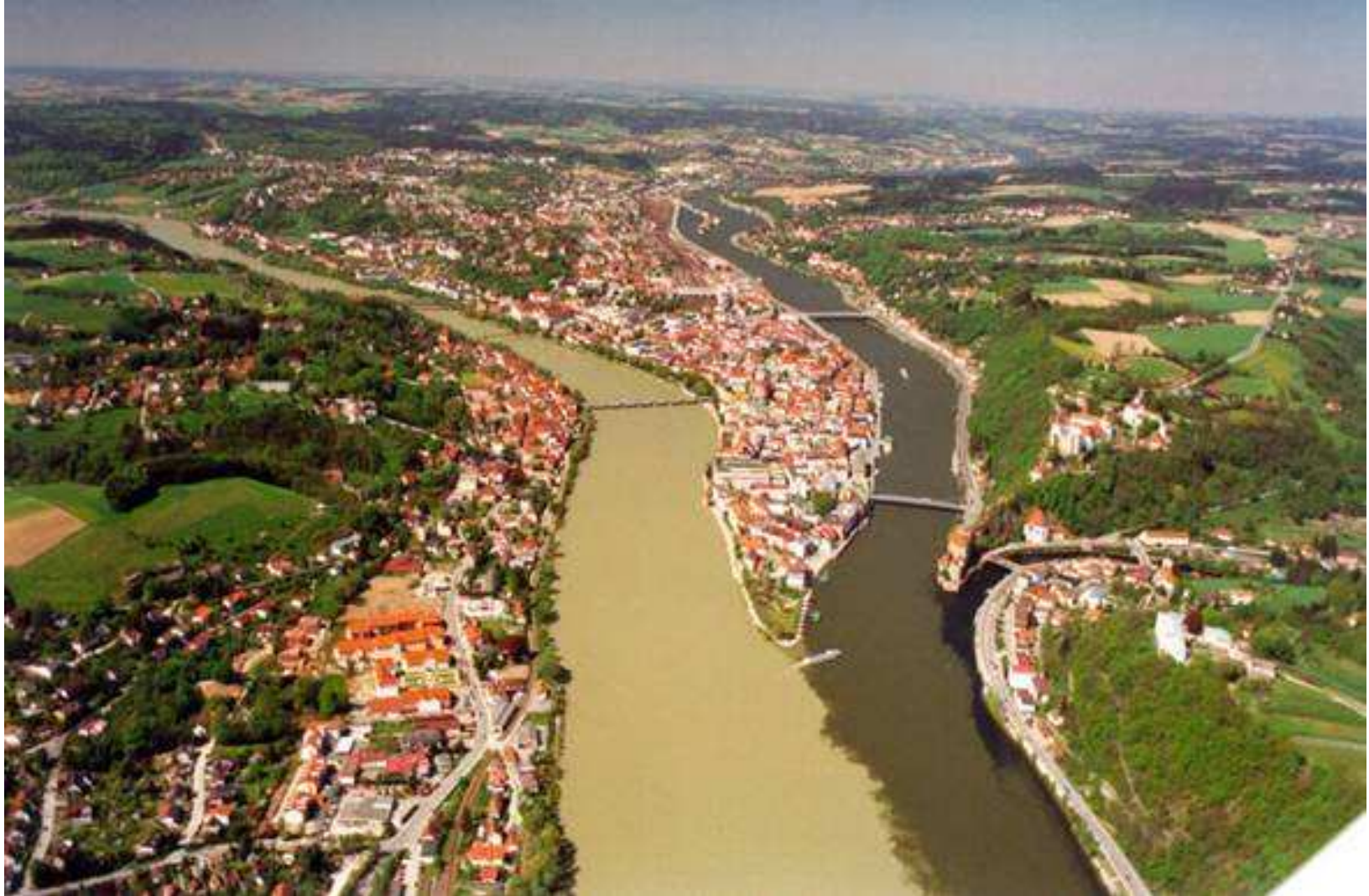
Laminar flow with low level of mixing.
