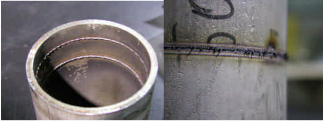
Figure 3 : Samples of weld and cut performed during the tests on the test bed
