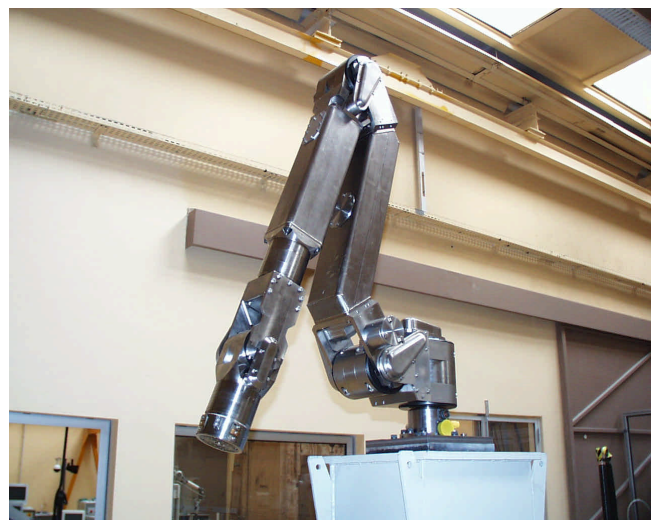
Figure 1 : The new Maestro manipulator commissioned at Fontenay-aux-Roses
