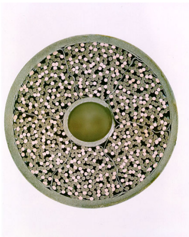
Figure 1 : TFMC conductor ( \Phi = 40.7 \text{ mm} )
