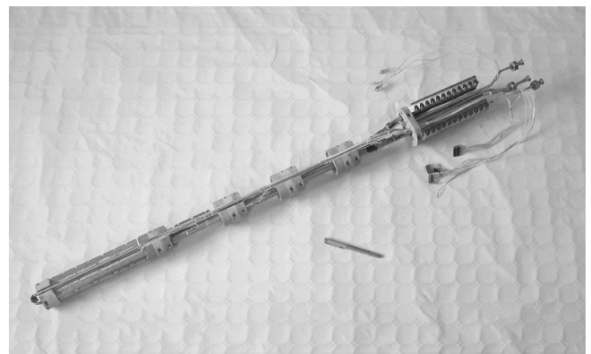
Figure 1 : Picture of a M50 sample showing the conductor joint on left and the bolt sample terminals on right (a pen is put for scale)
