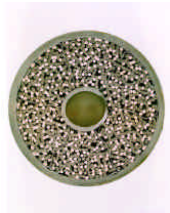
Figure 2 : TFMC CICC Cross section
