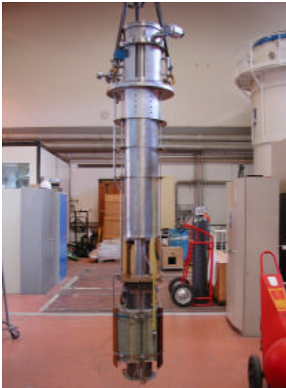
The upgraded JOSEFA sliding sample cryostat with the magnet at the bottom
