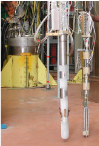
A subsize joint sample near its JOSEFA support The JOSEFA cryostat at the rear
