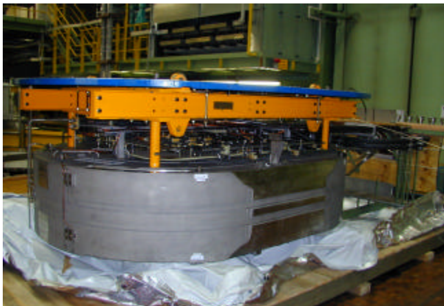
Figure 1 : TFMC delivered by AGAN at FZK (courtesy of FZK)
