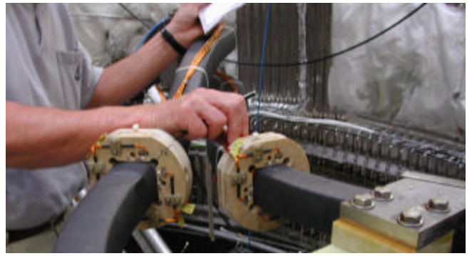
Figure 5 : Hall probes installed on the BB1 busbars
