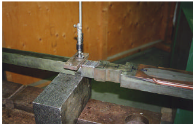
Figure 1 : Counter welds on the jacket of leg 2 near the upper termination
