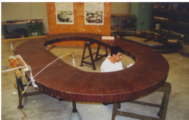
Figure 1 : TFMC double pancake completed
