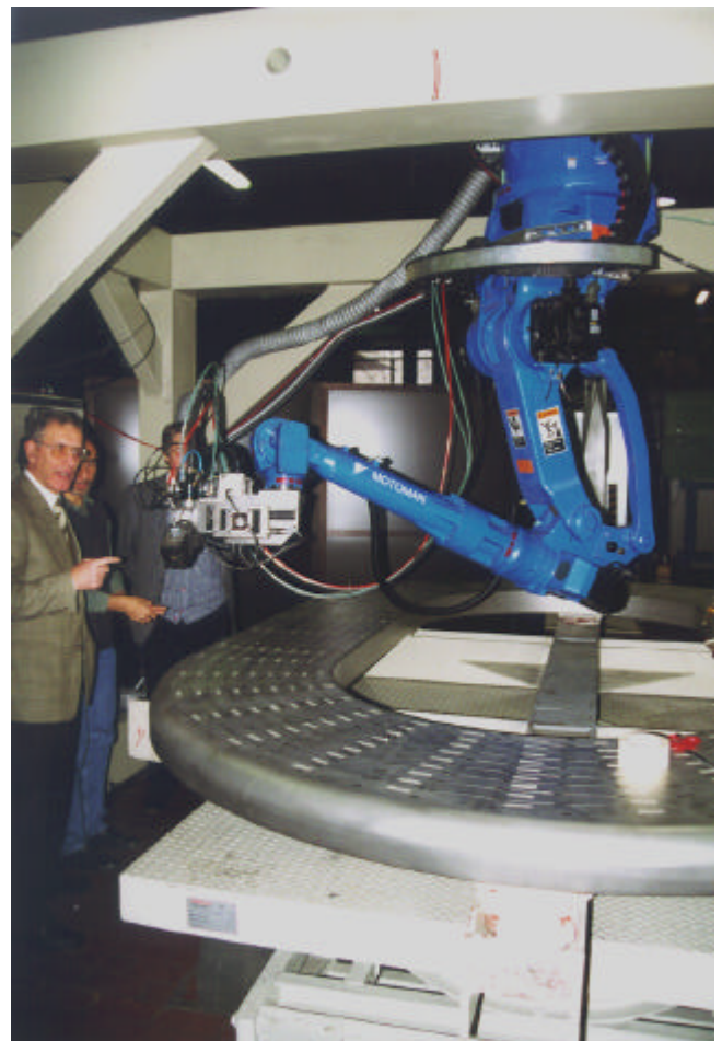
Figure 2 : Laser welding of TFMC radial plate covers
