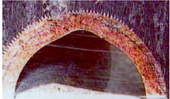
Figure 8 : Destructive examination of tile 12 after CHF, cross section BB on the side of tile 12
