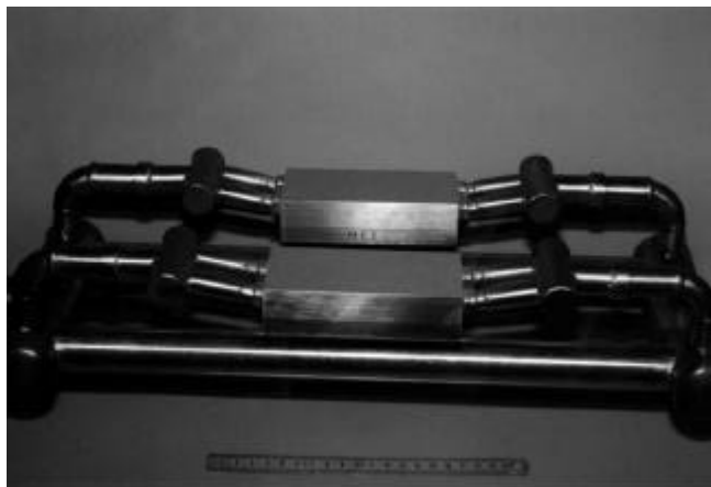
Figure 1 : MK1 and MK2 elements [CuCrZr (powder) Hipped to Stainless steel (powder and plate)] prepared for IR testing on SATIR
