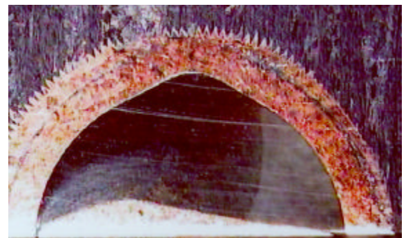
Figure 12 : Destructive examination of tile 12 after CHF, cross section BB on the side of tile 12
