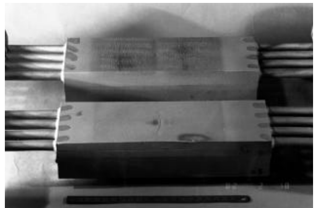
Figure 3 : FW2 mock-up after fatigue testing at 5 & 7 MW/m 2 . Disbonding failure on DS element and surface cracking on PH element
