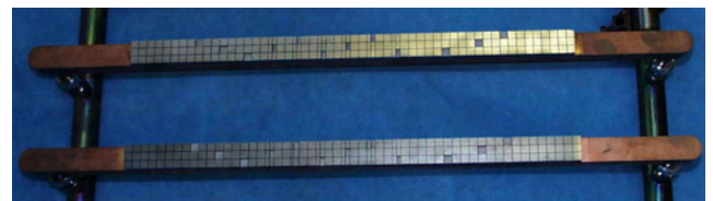
Figure 2 : The 2 W mock-ups W4 (upper) and W2 (down) assembled for HHF tests (armoured length = 460 mm)
