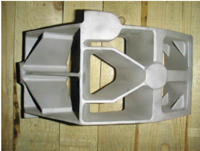
Figure 8 : Carrier mock up Inconel 650 vacuum cast & Hipped
