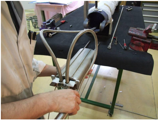
Figure 3: Segment assembly (First segment)
