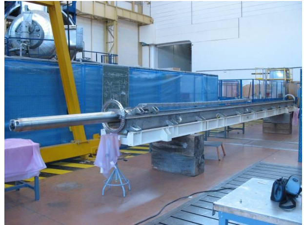
Figure 6: Storage cask, deployer and holding cable chain assembly
